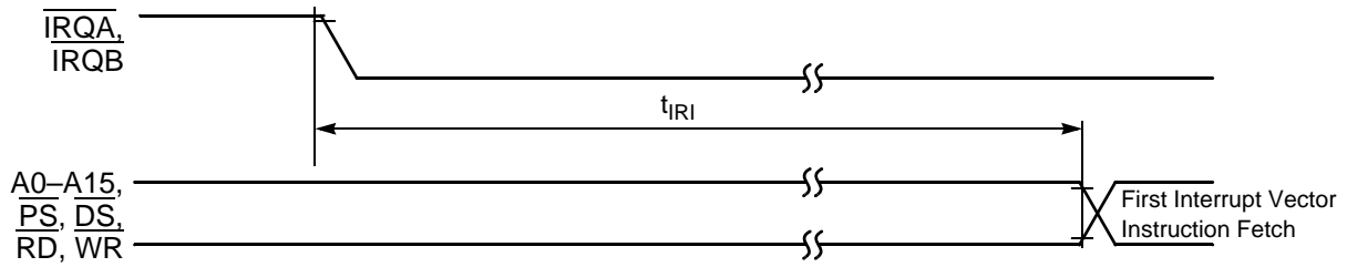
Figure 3-15 Interrupt from Wait State Timing
