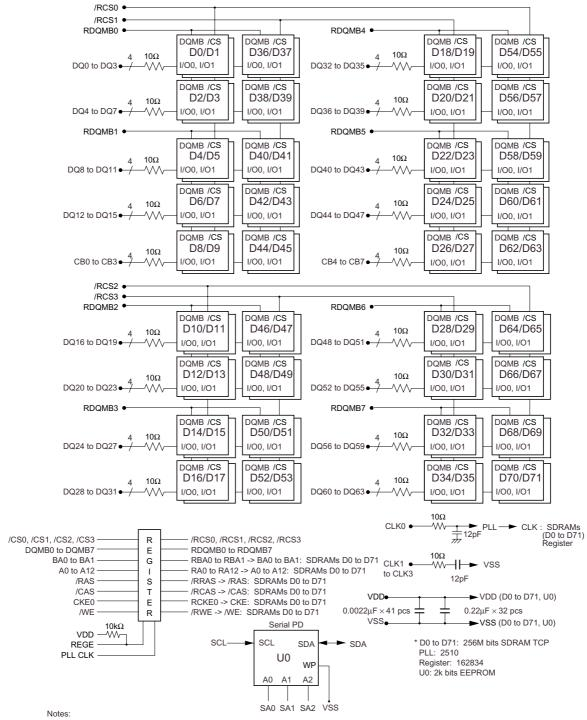
The SDA pull-up resistor is required due to the open-drain/open-collector output.
