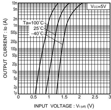
Fig.7 Output current vs. input voltage (OFF characteristics)
