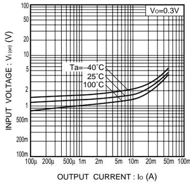
Fig.8 Input voltage vs. output current (ON characteristics)
