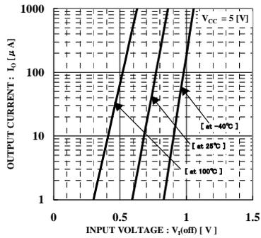
Fig.1 Output current vs. input voltage (OFF characteristics)
