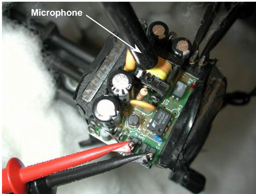
Figure 11. Test Arrangement for Audio Noise Measurement
