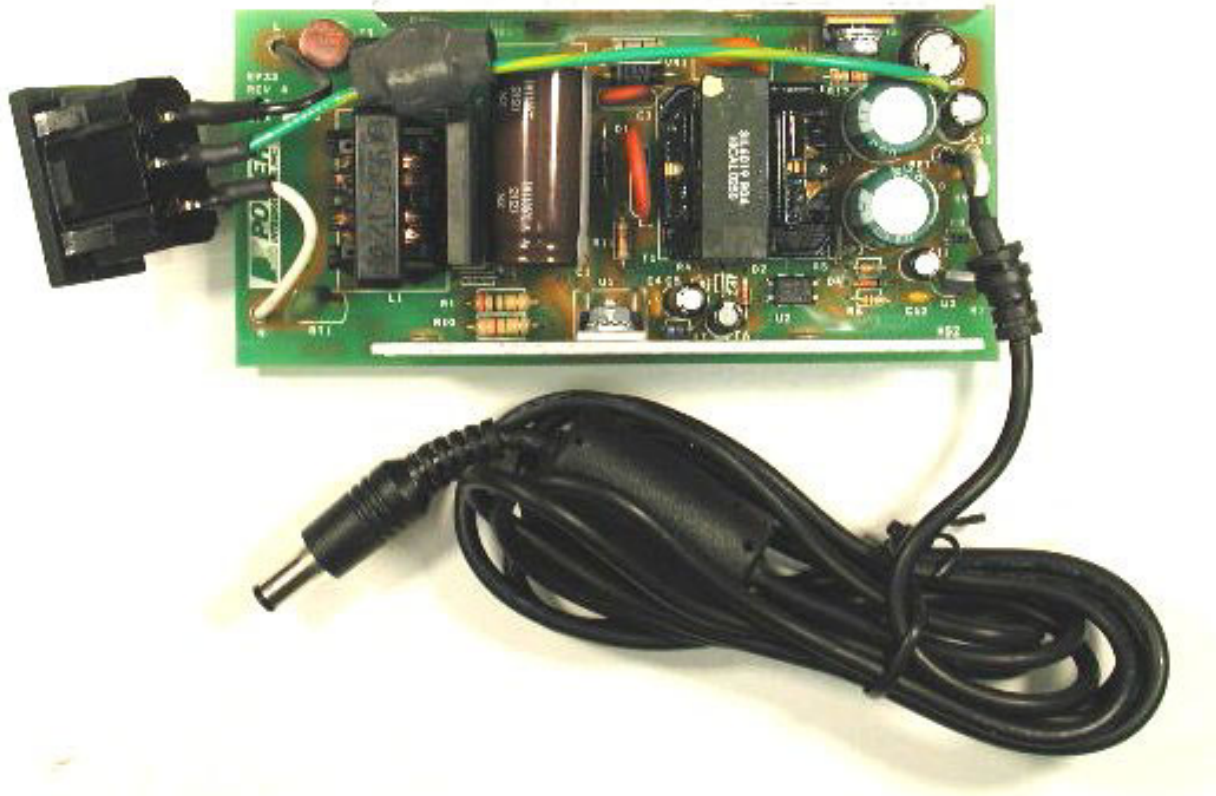
Figure 1 - EP-33 Populated Circuit Board.
