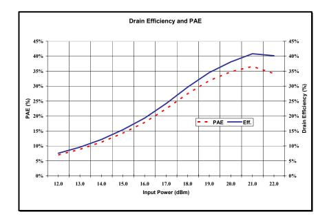
Typical power and efficiency is shown above. The devices were biased nominally at  $V_{DS} = 5V$ ,  $I_{DS} = 50\%$  of  $I_{DSS}$ , at a test frequency of 1.85 GHz. The test devices were tuned (input and output tuning) for maximum output power at 1dB gain compression.
