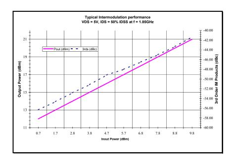
Note: pHEMT devices exhibit non-classical intermodulation performance, with equivalent IP3 values exceeding 14 dB above  $P_{1dB}$ . This IMD enhancement is affected by the quiescent bias current, the Drain-Source voltage, and the tuning or matching applied to the device.
