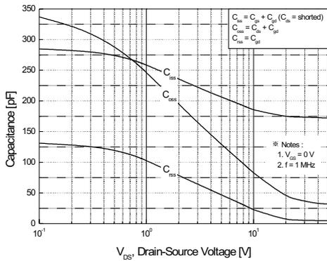
Figure 5. Capacitance Characteristics
