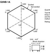
Quantity Tested: 5 units Test Method: Shock was applied 3 times in 6 directions along 3 axes and the level at which shock caused malfunction was measured. Rating: 100 m/s<sup>2</sup>
