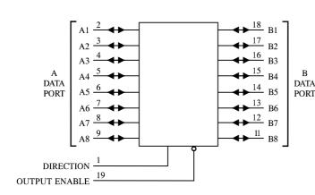
$PIN 20=V_{CC}$  PIN 10 = GND
