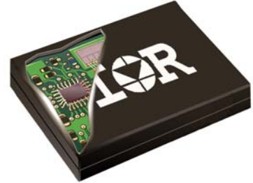
iP1202 Power Block
