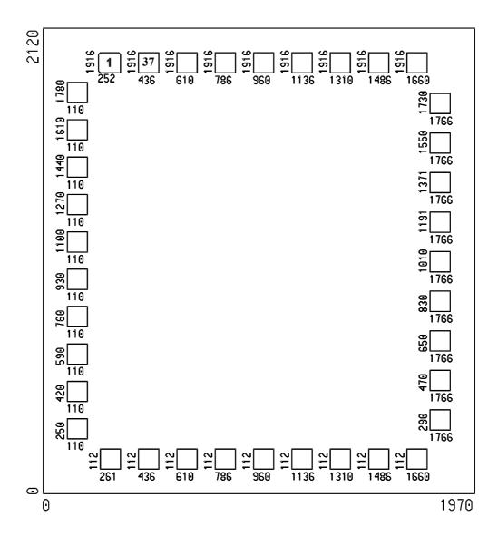
Chip size: 1.97 x 2.12 mm<sup>2</sup> \* The IC substrate should be connected to VDD in the PCB layout artwork.
