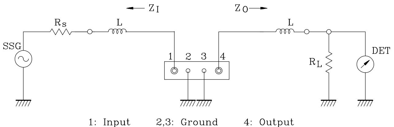
$R_S, R_L : 50\Omega$  (Internal Impedance of Source and Load)
