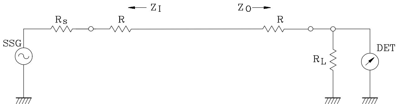
$R_S, R_L : 50\Omega$  (Internal Impedance of Source and Load)
