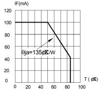
FIG.4 MAXIMUM FORWARD DC CURRENT VS
