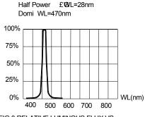
FIG.3 RELATIVE LUMINOUS FLUX VS. WAVELENGTH.
