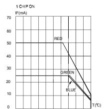
MAXIMUM FÖRWARD DC CURRENT VS, SOLDER POINT TEMPERATURE.
