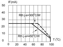
FIG.5 MAXIMUM FORWARD DC CURRENT VS TEMPERATURE. DERATING BASED ON Tjmax=110°C
