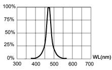
FIG.4 RELATIVE LUMINOUS INTENSITY VS. WAVELENGTH.
