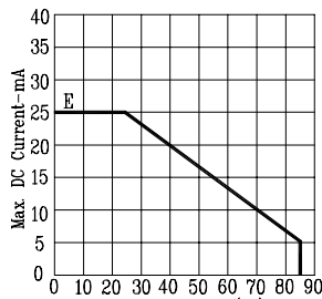
Fig5. MAX ALLOWABLE DC CURRENT VS. AMBIENT TEMPERATURE.
