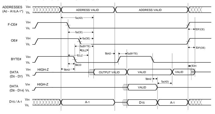
$When \ BYTE\#=VIH, \ F-CE\#=OE\#=VIL\ , \ D15/A-1 \ is \ output \ status. \ At this time, input \ signal \ must \ not \ be \ applied.$
