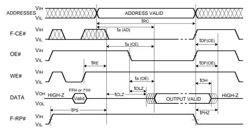
In the case of use F-CE# is Low fixed, it is allowed to define a timming specification of tRE from rising edge of WE# to falling edge of OE#, and valid data is read after spec of tRE+ta(CE). (This is only for FFH,71H program and read)
