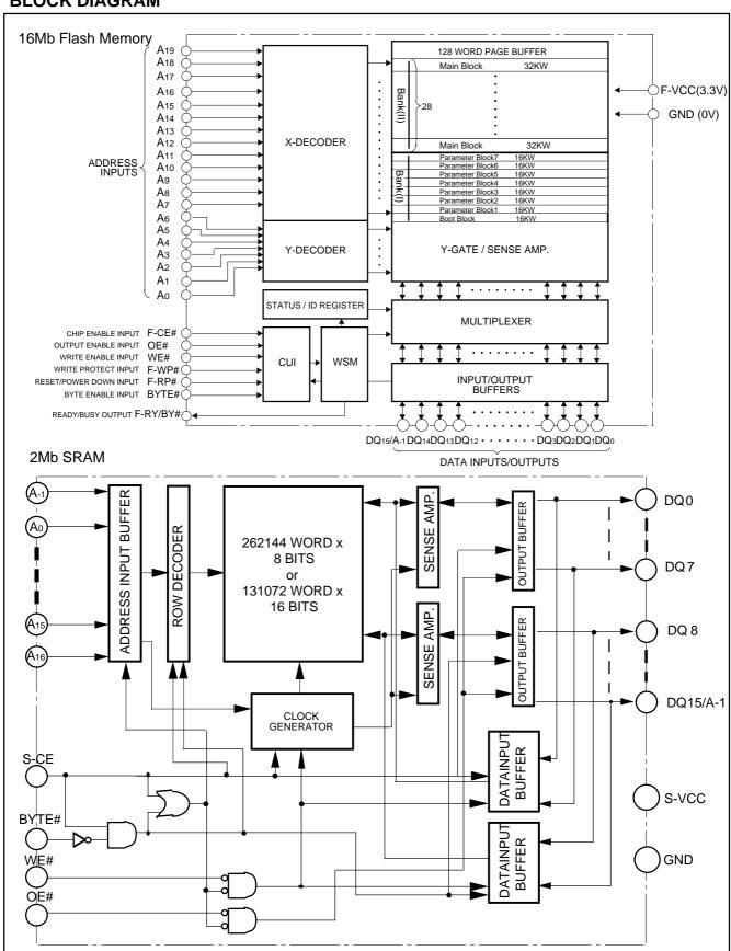
16,777,216-BIT (1,048,576 -WORD BY 16-BIT / 2,097,152-WORD BY 8-BIT) CMOS 3.3V-ONLY FLASH MEMORY & 2,097,152-BIT (131,072-WORD BY 16-BIT / 262,144-WORD BY 8-BIT) CMOS SRAM Stacked-MCP (Multi Chip Package)
