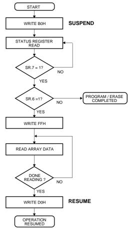
\* The bank address is required when writing this command. Also, there is no need to suspend the erase or program operation when reading data from the other bank. Please use BGO function.
