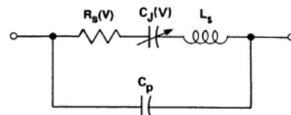
The **MA46H070 through MA46H073 (gamma 0.75)** family of constant gamma hyperabrupt GaAs tuning varactors has quality factor approaching that of abrupt junction varactors, but higher capacitance change versus tuning voltage. These diodes are very well suited for narrower bandwidth VCOs and VTFs where wide tuning range and very high quality factor are required.
