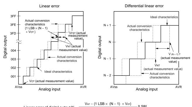
$$\label{eq:linear error} \text{Linear error of digital output N} = \frac{V_{NT} - \{1 \text{ LSB} \times \text{ (N-1)} + V_{OT}\}}{1 \text{ LSB}} \text{[LSB]}$$
