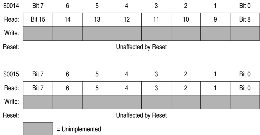
Figure 11-7. Input Capture Registers (ICRH and ICRL)
