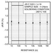
Fig.5 Resistance to soldering heat
