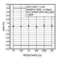
Fig.7 Damp heat, steady state
