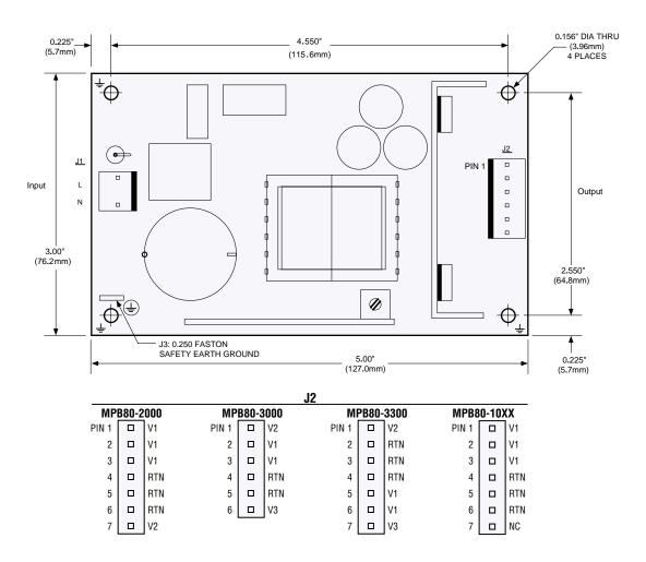
INPUT CONNECTIONS, J1: MOLEX 26-60-4030 OR EQUIVALENT HEADER MATES WITH MOLEX HOUSING 09-50-3031 OR EQUIVALENT AND PINS 08-50-0106 (18-20 AWG) OR 08-50-0108 (22-26 AWG) OR EQUIVALENT.
