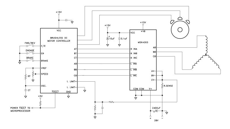
The MSK 4303 is designed to be used with a +28 volt high voltage bus, +15 volt low power bus and +5 volt logic signals. Proper derating should be applied when designing the MSK 4303 into a system. High frequency layout techniques with ground planes on a printed circuit board is the only method that should be used for circuit construction. This will prevent pulse jitter caused by excessive noise pickup on the current sense signal or the error amp signal.
