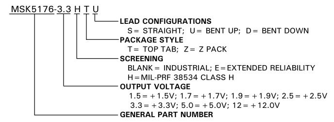
The above example is a +3.3V, Military regulator using the top tab package with leads bent up.
