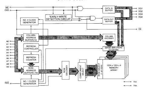
\*NOTE: 1. WE LOW prior to CAS LOW, EW detection circuit output is a HIGH (EARLY-WRITE)
