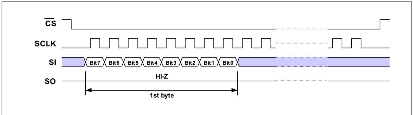
When incorrect command is inputted to this LSI, this LSI becomes standby mode and keeps the standby mode until next  $\overline{CS}$  falling edge. In standby mode, SO pin of this LSI should be High-Z. While  $\overline{CS}=VIH$ , current=standby current, while  $\overline{CS}=VIL$  and commands are issuing, or commands are invalid, current=5mA(typ.) to 15mA(max.).
