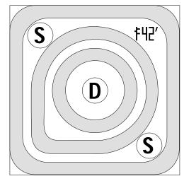
Die Size = 0.032" X 0.032" All Bond Pads = 0.004", Dia. Substrate is also Gate.
