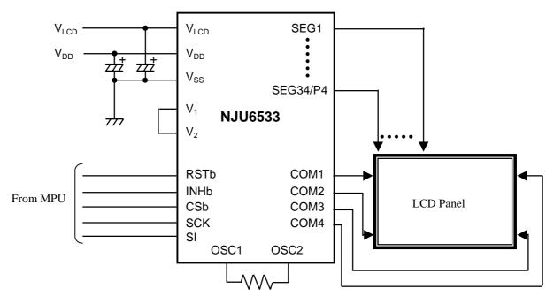
Note) Because display data is not yet stable just after V<sub>DD</sub> on, if LCD panel is turned on, unexpected pattern will be displayed, therefore, keep INHb terminal to "L" level until data transfer from MPU is over.
