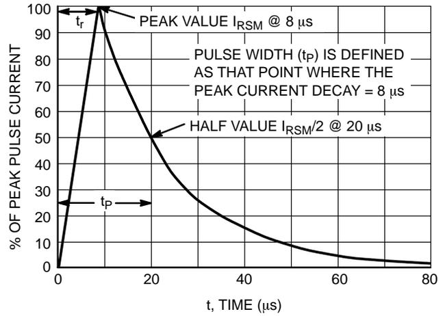
Figure 2.  $8 \times 20 \mu\text{s}$  Pulse Waveform
