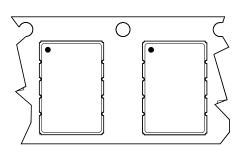
**Orientation in Tape Carrier as Shipped**
