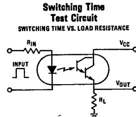
NOTE: Rise Time ( $t_r$ ) is time required for collector current to increase from 10% to 90% of its final value. Fall Time ( $t_f$ ) is time required for the collector current to decrease from 90% to 10% of its initial value.
