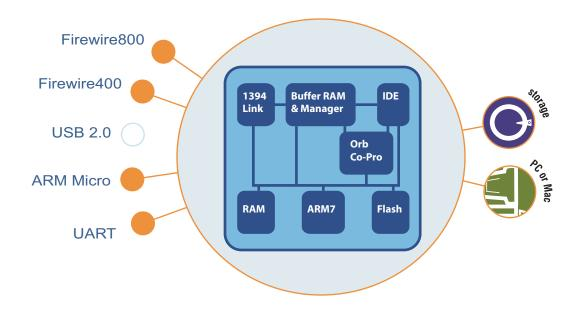
**The Oxford 912** is the latest generation 1394B (Firewire800) to ATA7/ATAPI (IDE) bridge. It supports all PIO, DMA and UDMA modes up to UDMA6, delivering a sustained data transfer performance of over 88MBytes/sec. Hardware features include SBP2.0 acceleration with 'fast start', in addition to dual disk striping and transparent spanning capabilities, all designed to achieve maximum data throughput on Firewire800.
