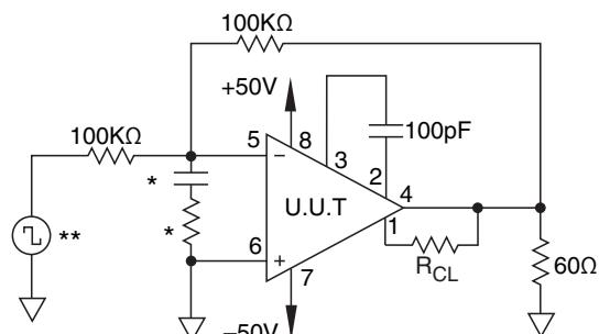
\* These components are used to stabilize device due to poor high frequency characteristics of burn in board.
