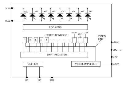
Figure 2. PI240MC-A4 Module Block Diagram
