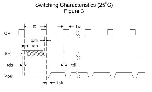
MODULE TIMING DIAGRAM
