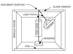
INSIDE PICTORIAL OF MODULE Figure 1. PI240MC-A4 Cross Section
