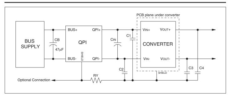
Figure 6 – Recommended schematic for QPI. Values of CIN and C1-C4 should be the values recommended by the converter manufacturer. If the manufacturer does not specify a value for the Y-capacitors use 4.7nF.  $Ry=10\Omega$ , 1/4 W.
