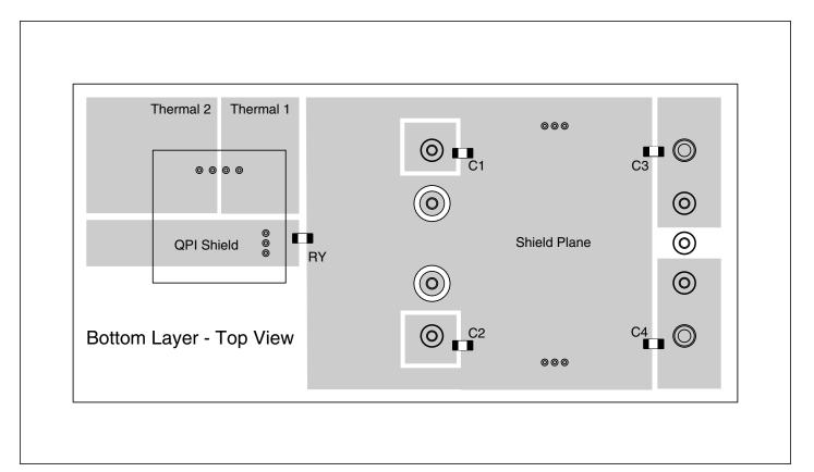
Figure 10 – Recommended layout for bottom layer of PCB. Note location of RY.
