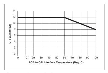
Figure 5 – QPI-2 current derating curve.
