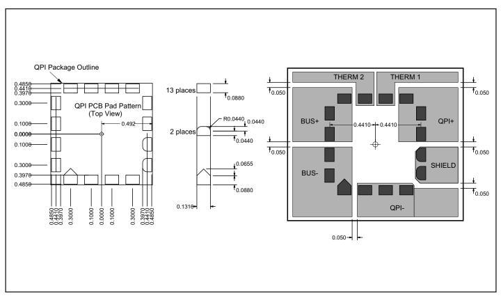
Figure 12 – Recommended PCB layout pattern. Use 1.3mm clearance around shield pads 5 & 6 to adjacent lands. See Figures 9 & 10 for recommended connection layouts.
