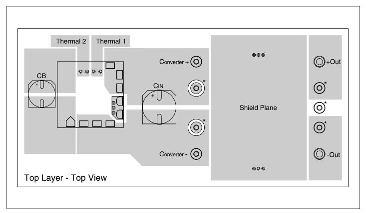
Figure 9 – Recommended layout for top layer of PCB. Pattern shows optional pins (\*) dependent on converter used in design. (Actual size with half brick footprint)
