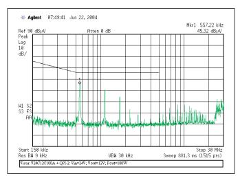
Figure 4 – Conducted EMI profile of a DC-DC Converter with OPI-2.
