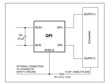
Figure 1 - QPI-2 circuit on input bus.
