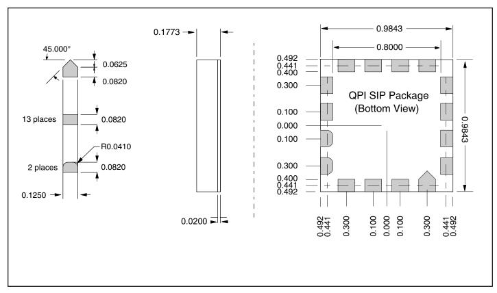
Figure 11 – QPI package dimensions and pad locations.
