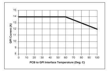
*Figure 5 – QPI-6 current derating curve.*
