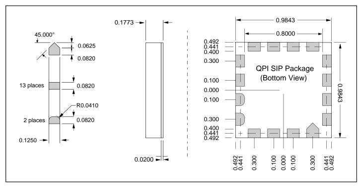
Figure 11 – QPI package dimensions and pad locations.
