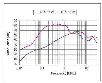
**Figure 2** - Attenuation curves showing common-mode and differential-mode attenuation.
