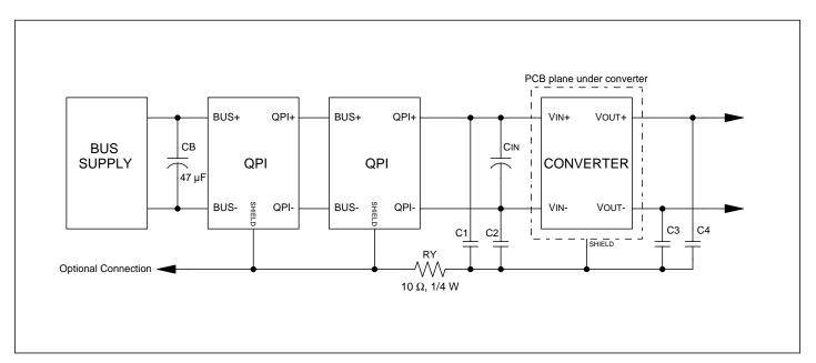
Figure 8 – Series connection of QPI for higher attenuation.
