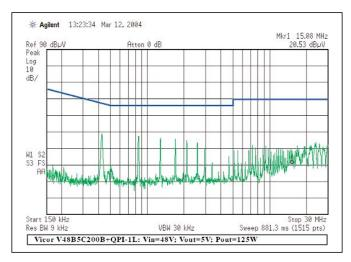
Figure 4 – Conducted EMI profile of a DC-DC Converter with OPI-6.
