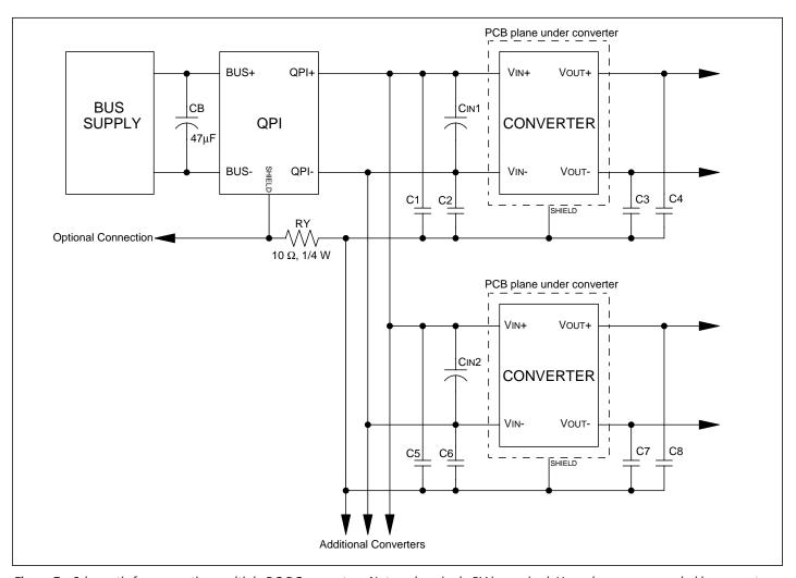
Figure 7 – Schematic for supporting multiple DC-DC converters. Note only a single RY is required. Use values recommended by converter manufacturer for CIN and Y-capacitors C1-C8.
