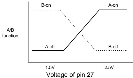
**NOTE:** The voltage of pin 27 is forced by a switch controller. If the voltage varies very fast from low to high, or high to low, then tape output makes a large pop noise.
