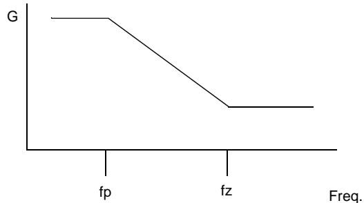
$$f_p = \frac{1}{2\pi(R_1 + R_Z)C_1} \quad f_z = \frac{1}{2\pi R_Z C_1}$$
