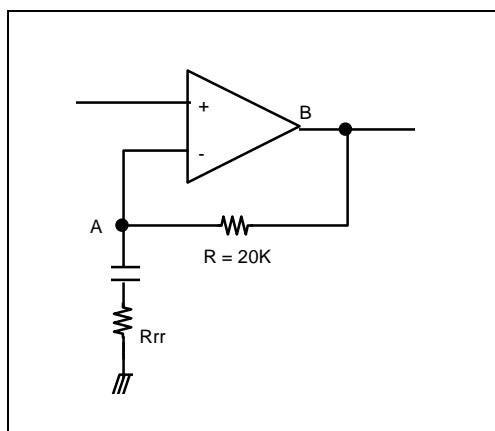
Point A is pin 2 and pin 35, B is pin 44 and pin 42.
