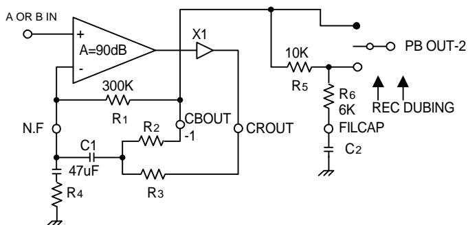
$$H_{NAB}(S) = \frac{\frac{1}{S + \frac{R_Z C_1}{1}}}{\frac{1}{S + \frac{(R_1 + R_Z) C_1}{1}}} \quad R_Z = R_2/R_3: \text{Cro MODE}$$
