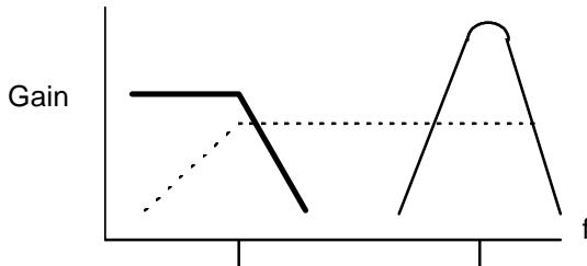
Internal part  $R_{M3}$  and external  $C_L$  are fixed and  $R_{GM}$  is adjustable by means of the external. Hence, gain of mid and low frequency are controlled.
