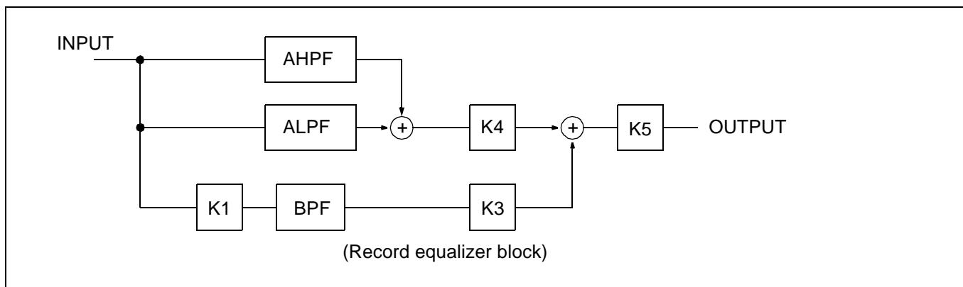
If  $K_5$  is 10, the record maximum output level is 1 Vrms and the output noise is 0.8 mVrms. We recommend that you keep it between 10 and 20 if possible.
