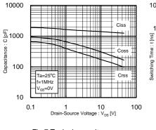
Fig.7 Typical capacitance vs. Source-Drain Voltage
