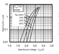
Fig.1 Typical Transfer Characteristics
