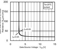
Fig.5 Static Drain-Source On-State Resistance vs. Gate-Source Voltage
