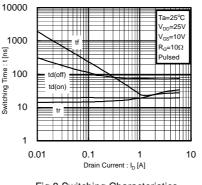
Fig.8 Switching Characteristics
