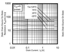
Fig.4 Static Drain-Source On-State Resistance vs. Drain Current (3)
