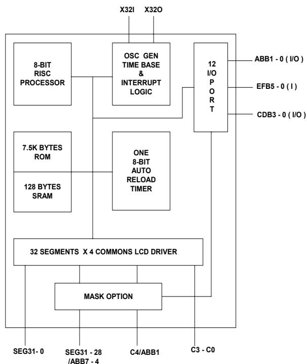
**Note1:** By mask option, SEG31 - 28 can be defined as either segment output or I/O. (SEG31 - 28 or ABB7 - 4)
