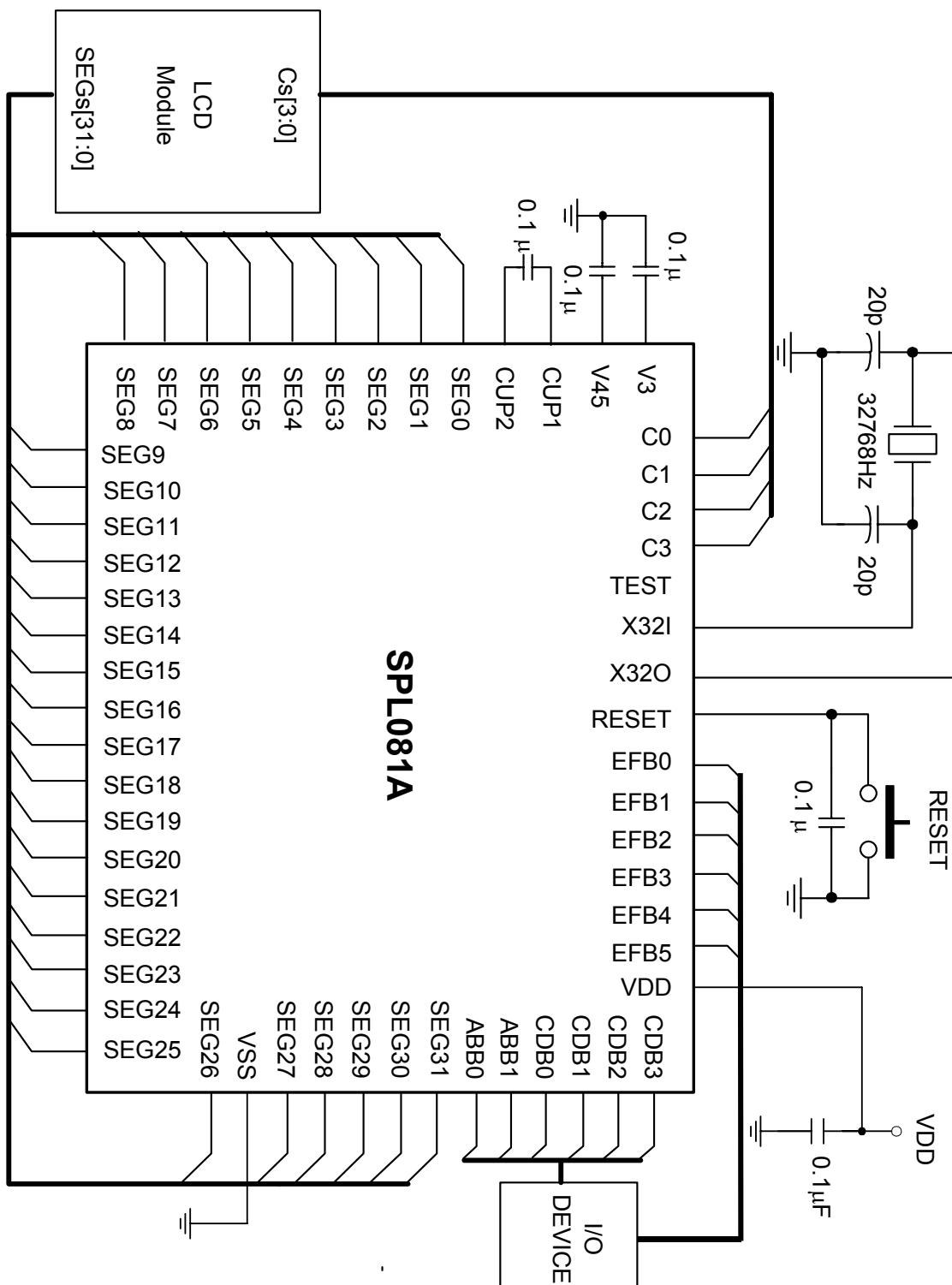
Note: The 0.1μF capacitor between VDD and VSS should be placed to IC as close as possible.
