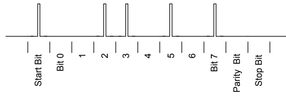
FIGURE 18-3 IrDA ASCII “S” with Odd Parity
