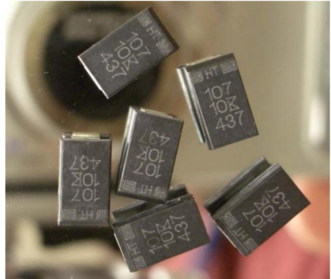
Figure 2. Photograph of "D" case, T498 SMT capacitors.
