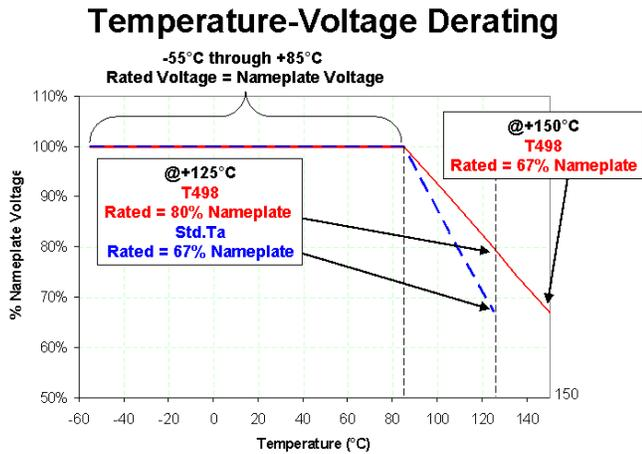
Figure 4. Voltage-temperature derating for standard and T498 capacitors.
