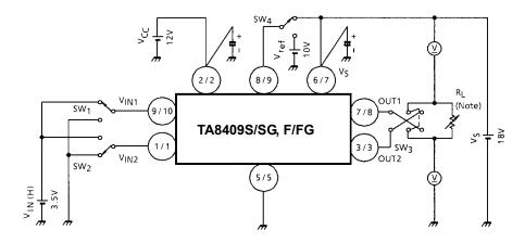
Note: Calibrate I<sub>OUT</sub> to 0.2/0.4 A by R<sub>L</sub>.
