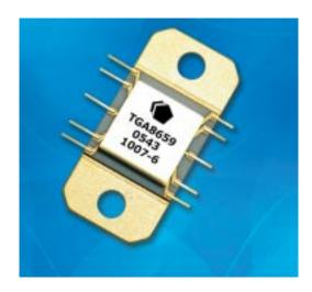
The TriQuint TGA8569-FL is a packaged Power Amplifier delivering more than 4 Watts in the VSAT Band. The power amplifier works over the extended frequency range of 13 to 17 GHz and is designed using TriQuint's proven standard 0.5 um gate pHEMT production process.
