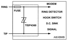
Figure 16. MODEM INTER-WIRE PROTECTION
