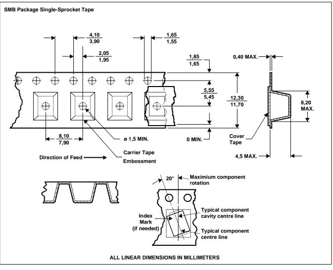
NOTES: A. The clearance between the component and the cavity must be within 0,05 mm MIN. to 0,65 mm MAX. so that the component cannot rotate more than 20° within the determined cavity. MDXXBJ
