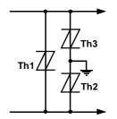
Figure 11. TWO POINT PROTECTION
