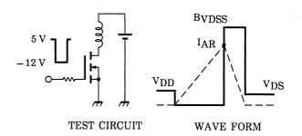
$$\begin{array}{l} T_{ch} = 25^{\circ}C \; (Initial) \\ Peak \; I_{AR} = -5 \; A, \; R_G = 25 \; \Omega \end{array} \quad E_{AS} = \frac{1}{2} \cdot L \; \cdot I^2 \cdot \; (\frac{B_{VDSS}}{B_{VDSS} - V_{DD}}) \\ V_{DD} = -16 \; V, \; L = 1.0 \; mH \end{array}$$
