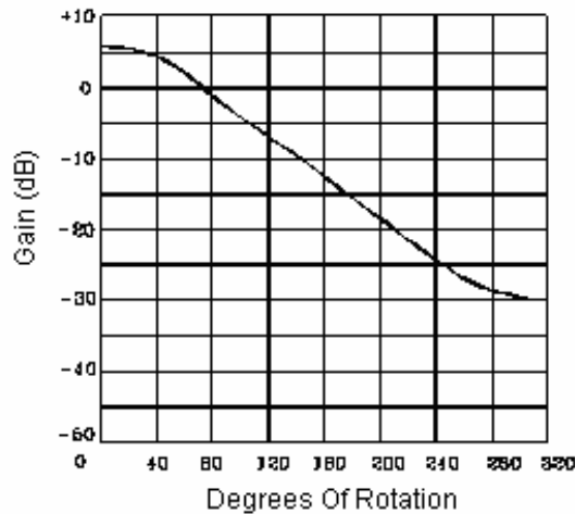
Figure 12. Receive Attenuator Gain versus Potentiometer Position Using Audio Taper
