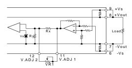
Resistance values when adjusting output voltage (Equation 1)
