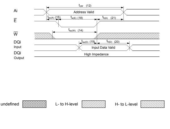
i: If  $\overline{W}$  is LOW and when  $\overline{E}$  goes LOW, the outputs remain in the high impedance state.
