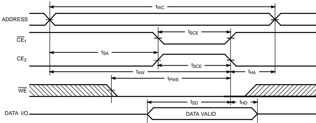
**Write Cycle No. 2 ( $\overline{WE}$  Controlled,  $\overline{OE}$  HIGH During Write)<sup>[10, 14]</sup>**
