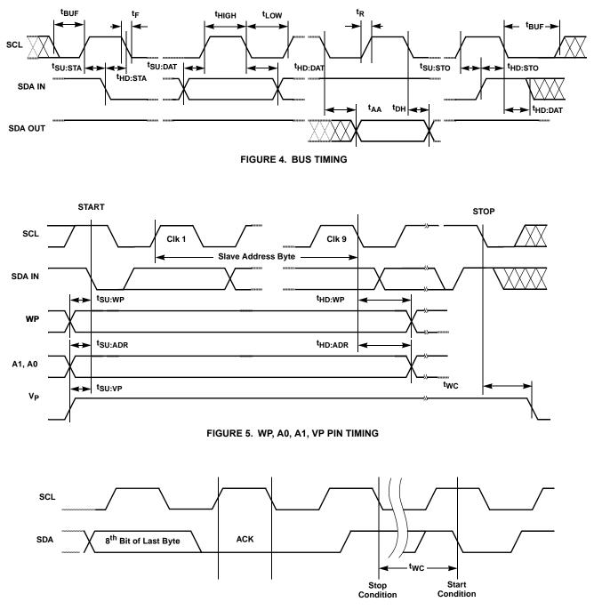
FIGURE 6. WRITE CYCLE TIMING
