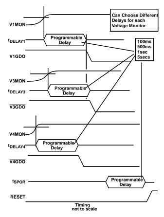
FIGURE 8. PARALLEL POWER CONTROL - TIMING
